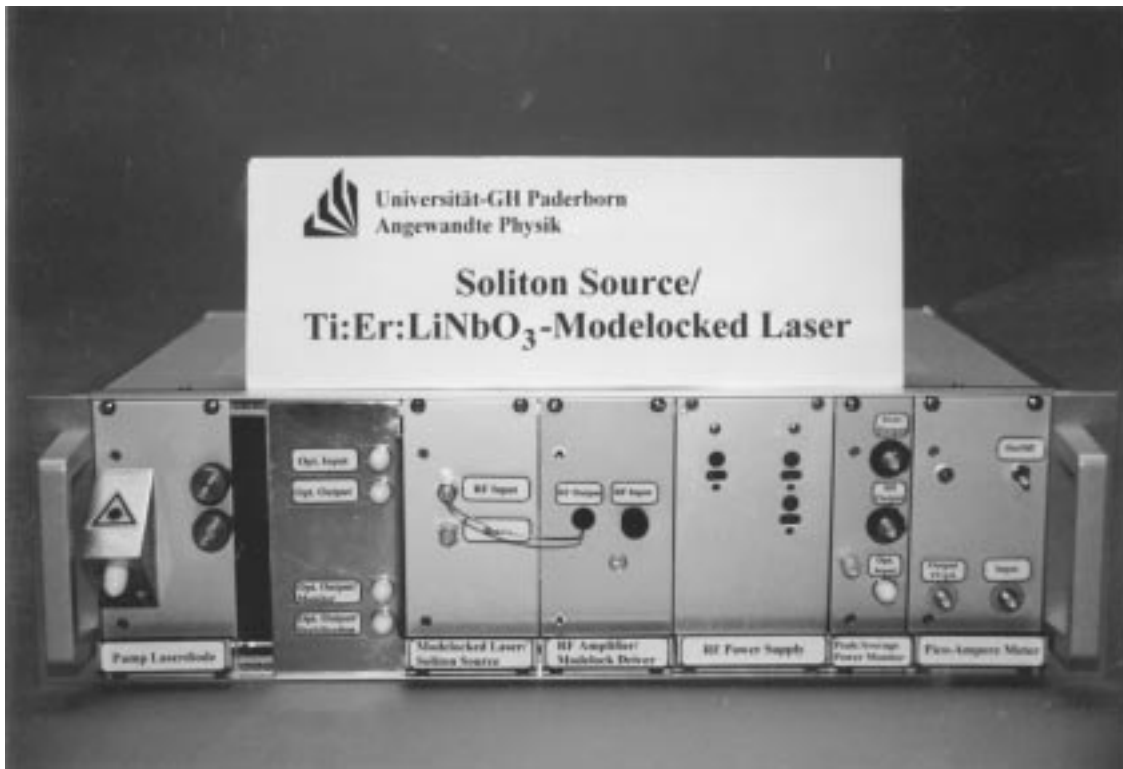
Fig. 3. Photograph of the rack-mounted, packaged soliton source (for more details see text).
