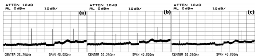
Fig. 3. RF Spectra at the (a) Output of the Compressor, (b) Output of the Fabry-Perot filter and (c) Output of the 40 GHz Pulse Source. Amplitude Scale is 10 dB/div and Frequency Scale is 4 GHz/div
