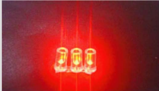
AlGaInP/GaAs RCLEDs emitting at 650nm. Note the forward-directed emission pattern similar to that of a semiconductor laser (courtesy of Osram Opto Semiconductors Corporation, Germany, 1999).
