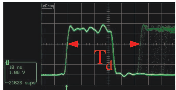
Figure 7. Typical output signal of an APD module [4], when it is operated at ‘high’ intensities. During the dead-time T_d no subsequent signal gets registered even though there are optical signals impinging on the diode.
