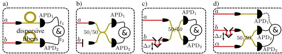
Fig. 5. Scheme of different measurement settings. a) JSI measurement; b)  $g^{(2)}(0)$  measurement; c) HOM interference between signal and idler; d) 2-fold or 3-fold HOM interference with a reference field. The Id Quantique detectors (1 MHz) are used for the JSI measurement and the NuCrypt detectors (40 MHz) for the rest.
